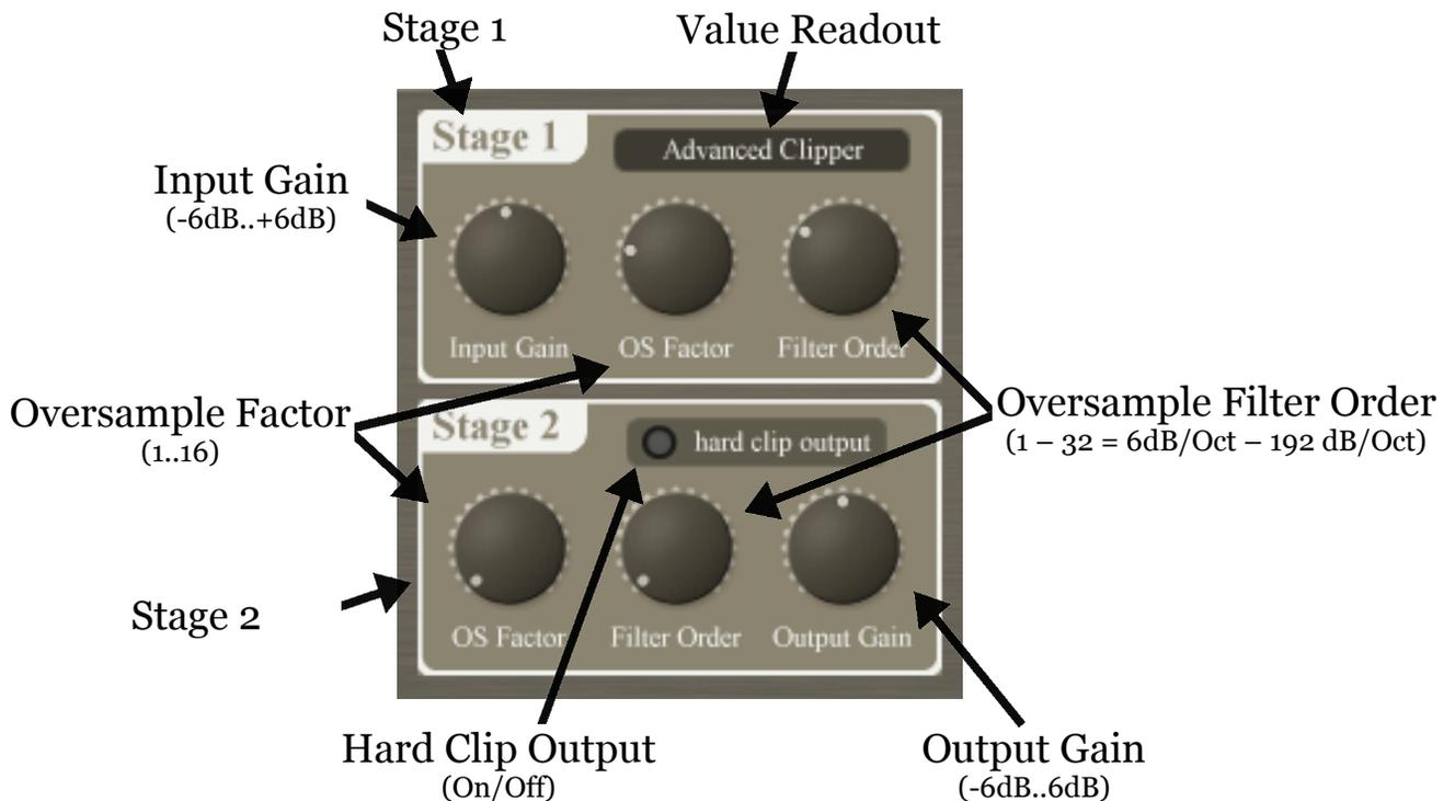
The plugin features 2 independent clipping stages and an additional hard clipper on the output. Each stage contains an adjustable oversampling filter. Furthermore in the first stage the input gain can be controlled and in the second stage the output gain can be controlled.
